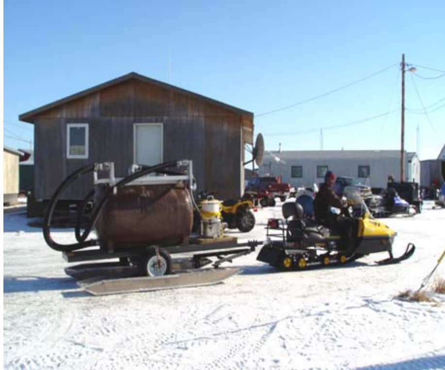
Photo 5: Roll-on Skis at work with sewage tank mounted. The sewage vacuum blower is mounted on the platform in front of the sewage tank.
