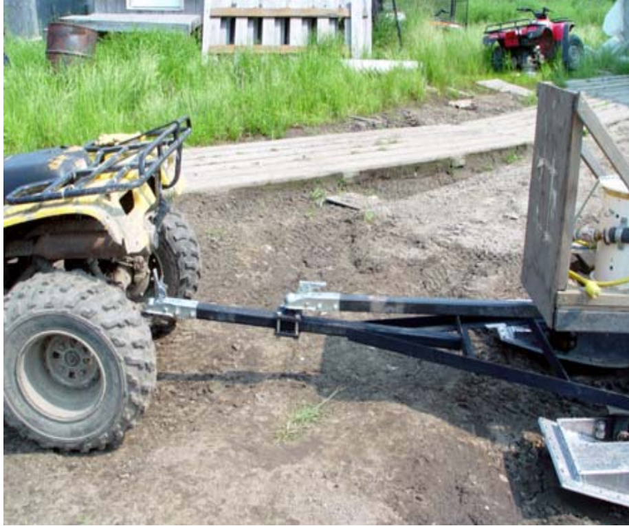
Photo 7: Easy hitch set-up for Roll-on Skis. Two simple ball hitches is all it takes to connect. The first one connects the skis to the tow vehicle. The second one connects the trailer to the tow bar of the skis.
