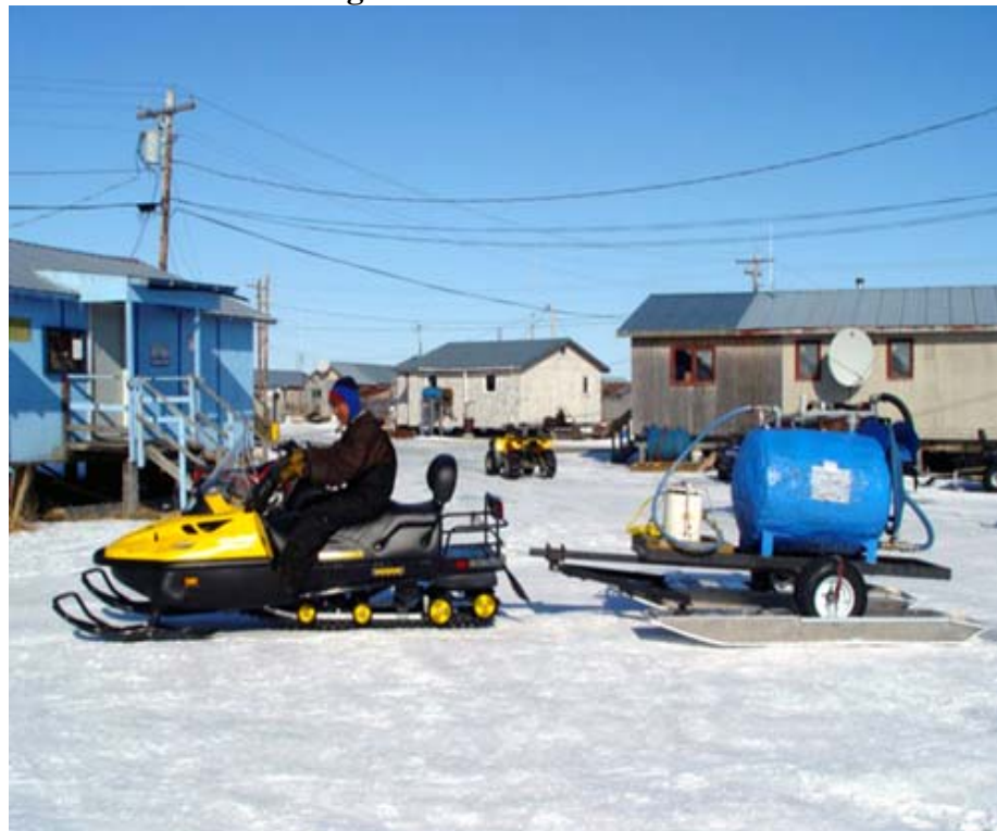
Photo 6: Roll-on Skis with water tank mounted. The water blower is mounted on the platform in front of the water tank
